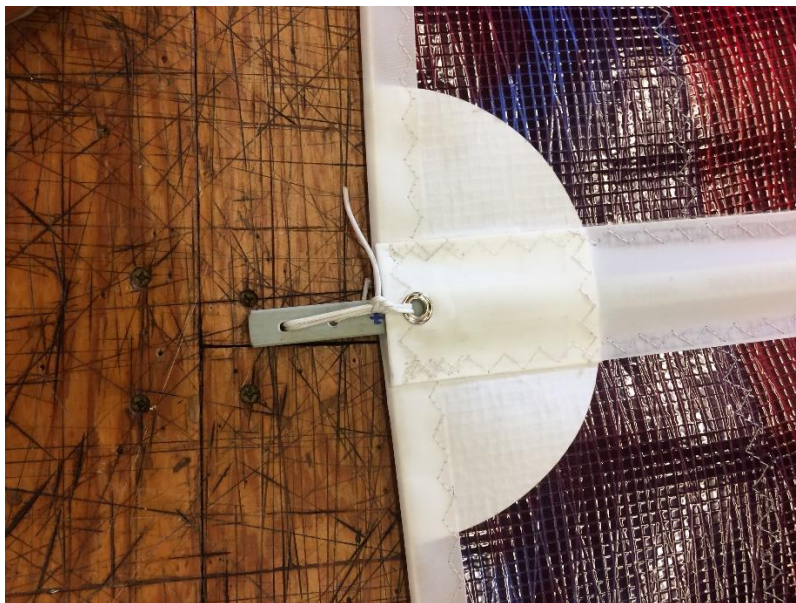
Figure 6 – Double and triple the leech line knot
