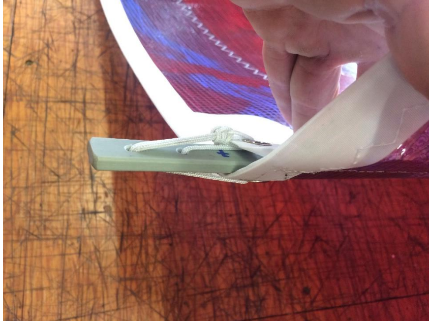
Figure 7 – Correct installation of a batten
