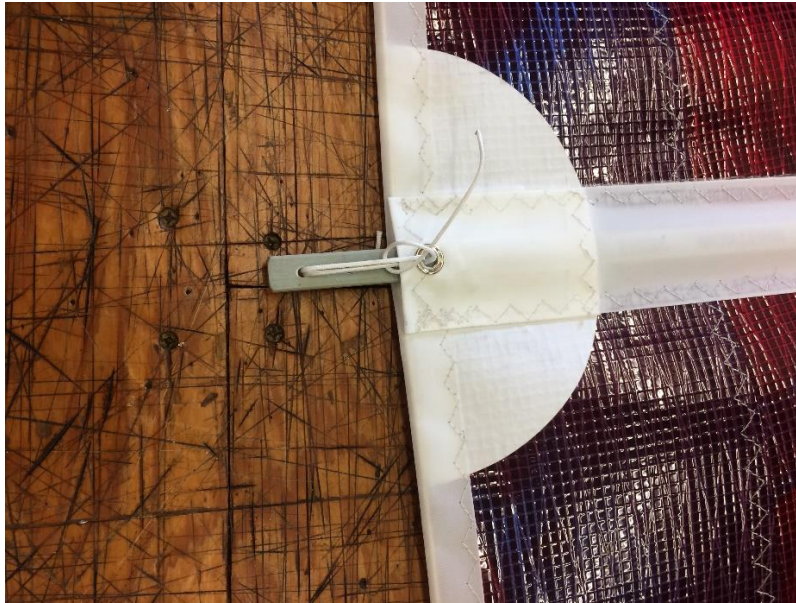
Figure 5- Tie a knot to keep leech line tight
