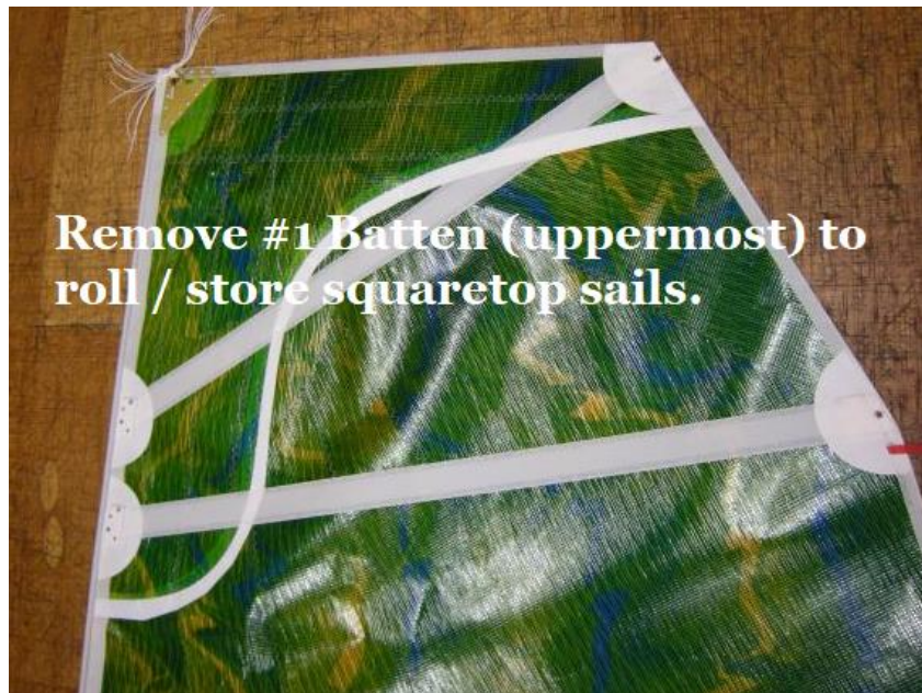
Figure 8 – Remove top batten to roll sail
