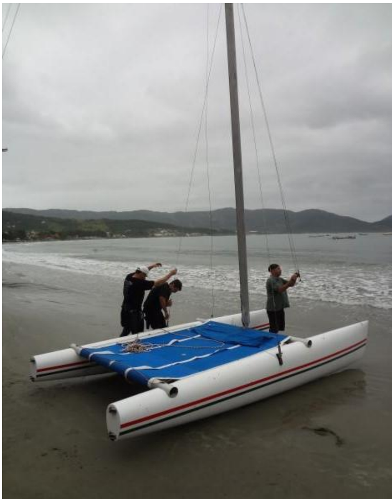
Super Cat 17 Double Wrap Example (Trampoline wraps both the forward and aft beam)
