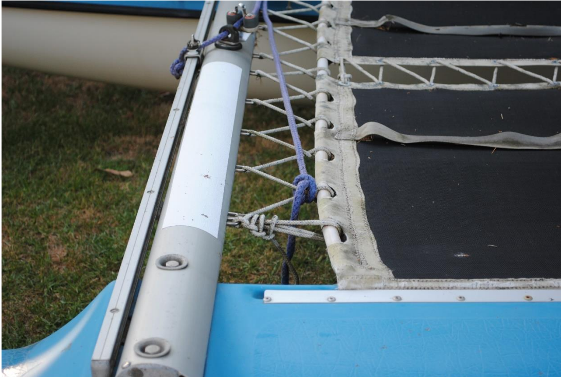
Maricat 4.3 center and aft lacing pattern and knots
