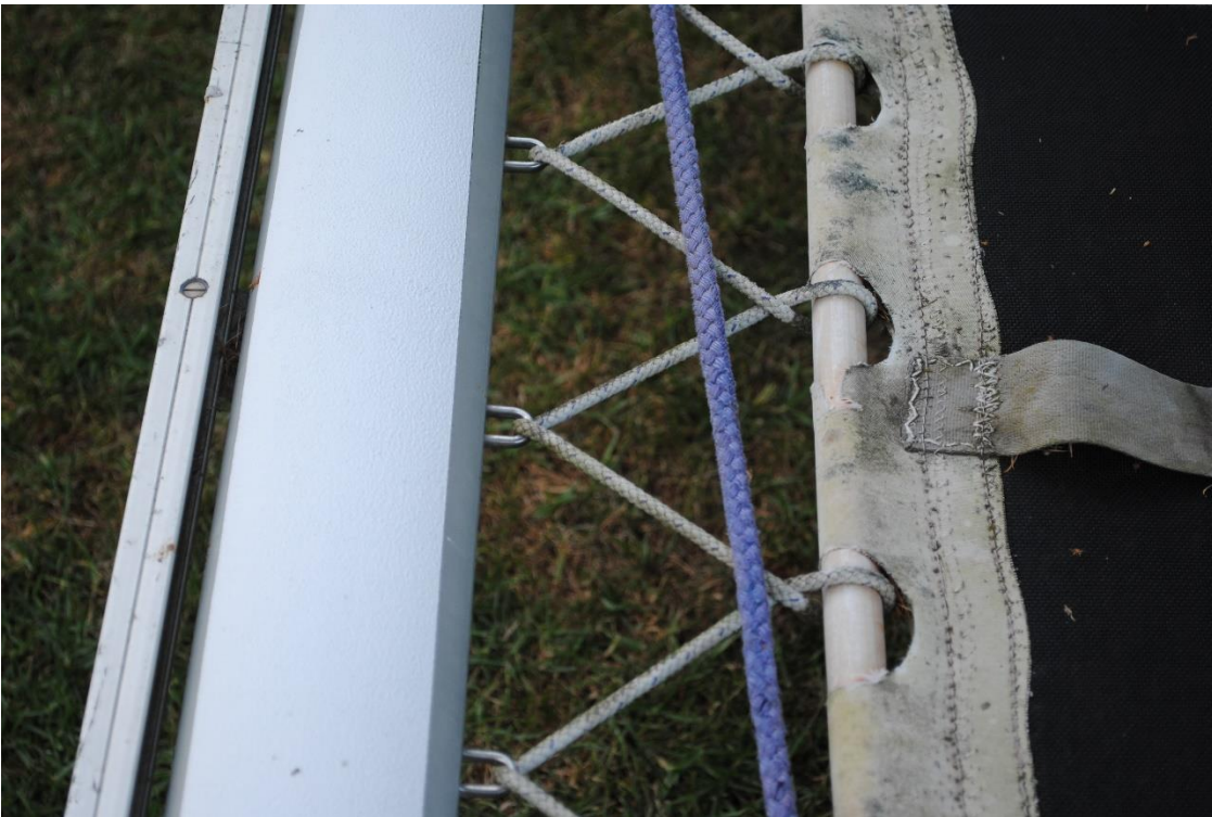
Maricat 4.3 aft beam's sail slides and PVC tube
