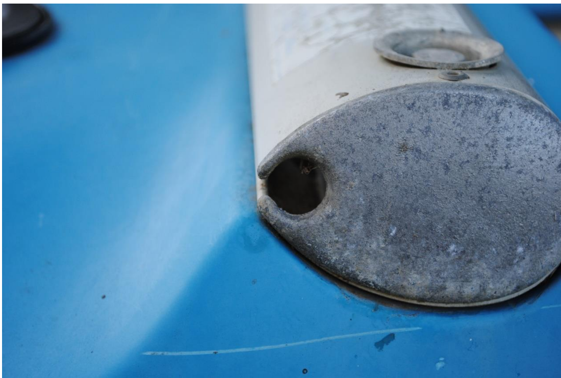
Maricat 4.3 front beam profile showing boltrope track
