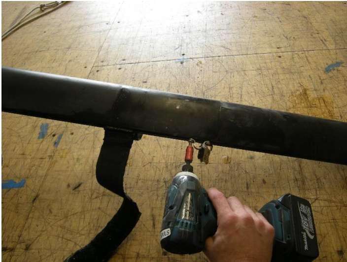
Figure 3 - Removal of rear cross beam eye strap
