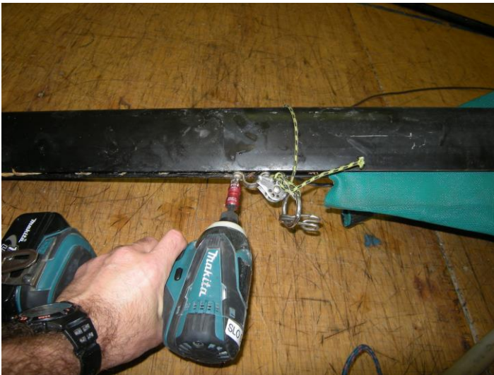
Figure 5 - Removal of forward cross beam eye strap
