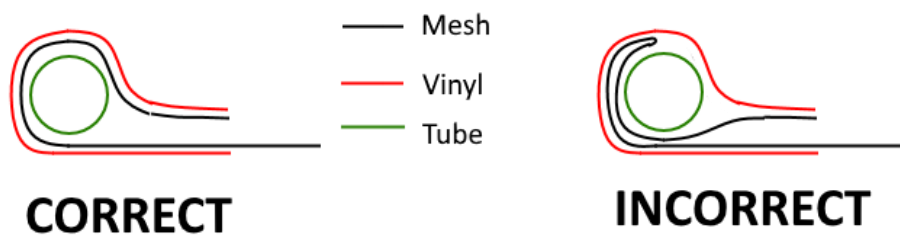
Figure 8 - Tube installation diagram
