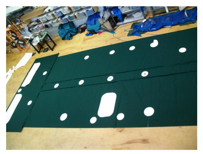
The above photo shows the number of reinforcements we add to our custom pontoon boat covers. We reinforce around all bimini top cutouts and mounting hardware as well as over the windshield and at each pole support. Any other places on the cover that may wear are also reinforced.
