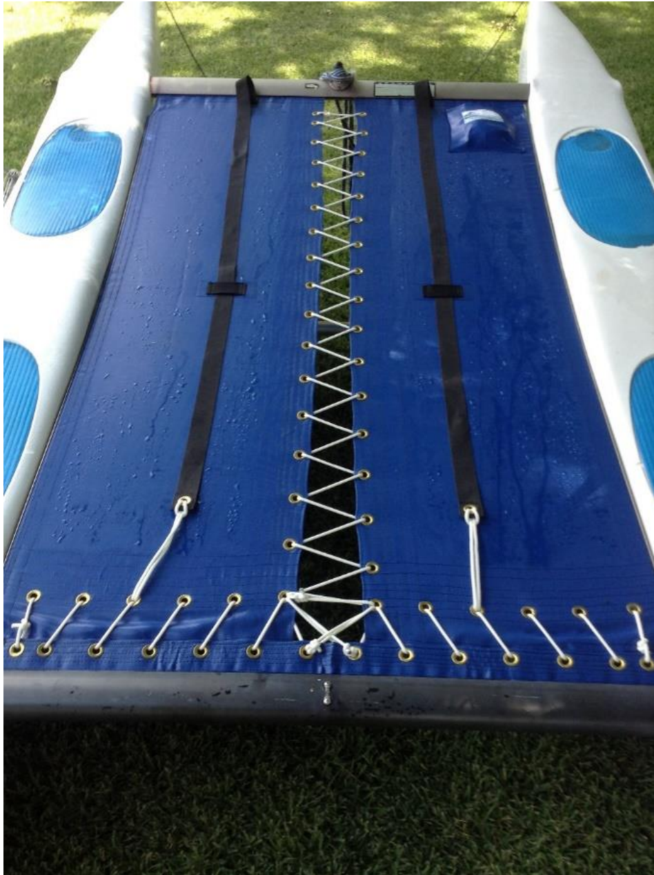
Figure 4 - Completed trampoline installation
