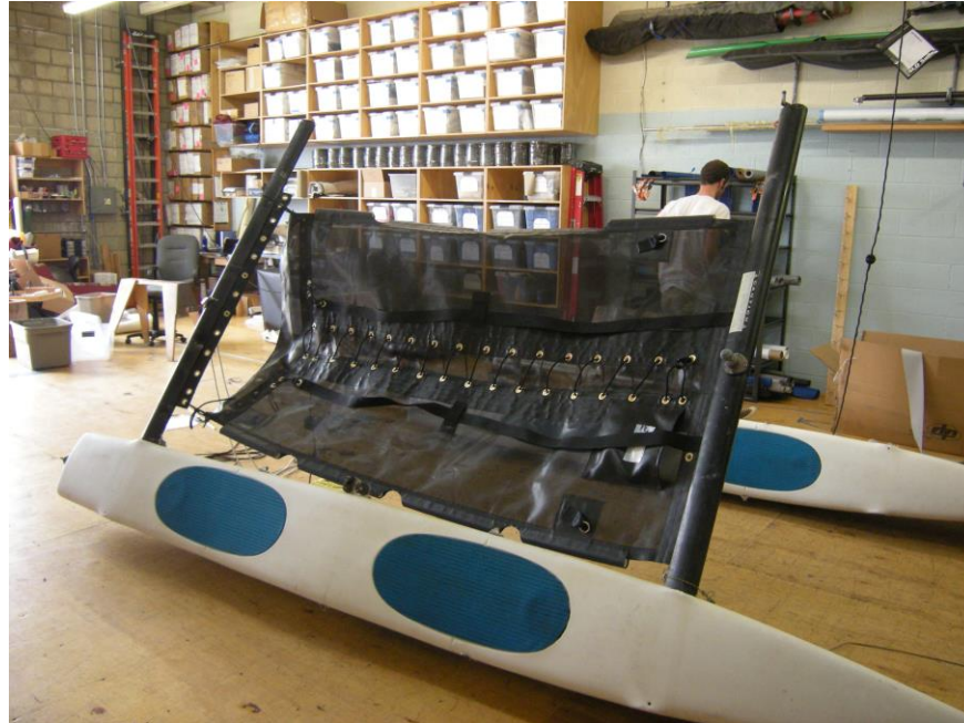
Figure 3 - Trampoline attached to cross beams
